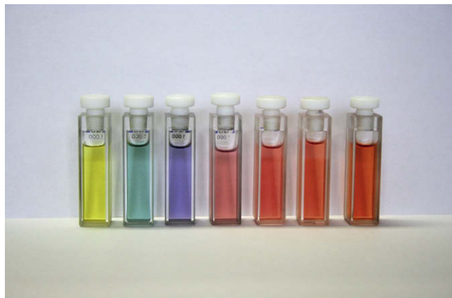
Figure 7. Compound 7 in acetonitrile solution ( 4 \times 10^{-5} M) and addition of several bases ( 6.6 \times 10^{-5} M); from left to right: 1 : without base, 2 : LiOH, 3 : NaOH, 4 : KOH, 5 : RbOH, 6 : CsOH, 7 : Et 4 NOH.
